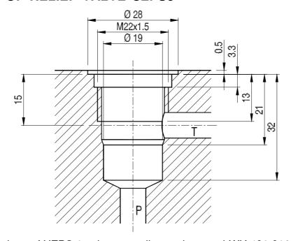
Detailed specifications of UZPS 6 valve according to data card WK 492 860
